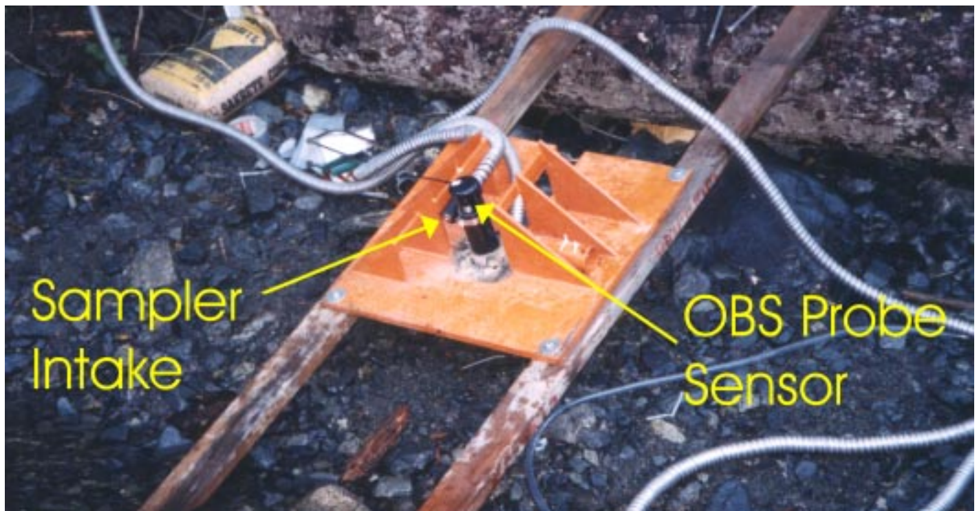
Figure 1. Steel-plate in-stream instrument mount; the OBS probe is mounted in the ABS pipe in the center of the plate. The sampler intake and the OBS sensor are 20 cm above the base of the plate. This assembly is placed in a stable pool in the channel. The plate must be placed on a stable bed with no large void spaces underneath, and weighed down with rocks to avoid being flipped by turbulent high-flow conditions.
