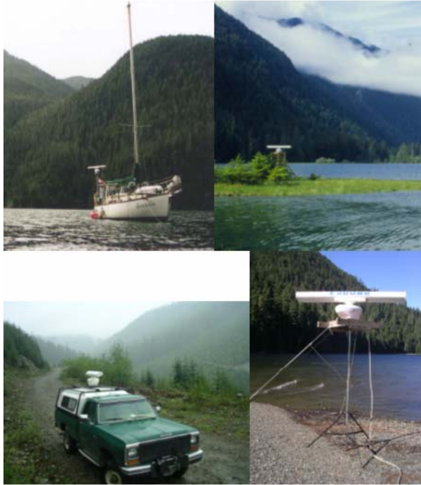
Figure 2. Boat, vehicle and land-based radar set-ups.
