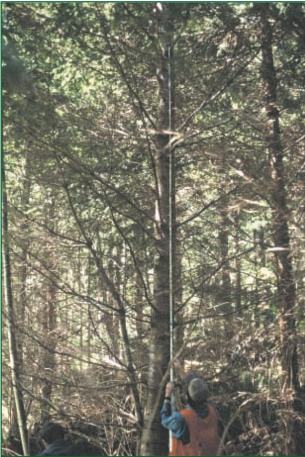
**Figure 1.** Telescoping height pole used to measure the past height of a site tree each year as it grew above bh, based on the location of branch whorls.
