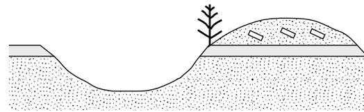
FIGURE 4. Furrow and berm prepared by disc trencher.
