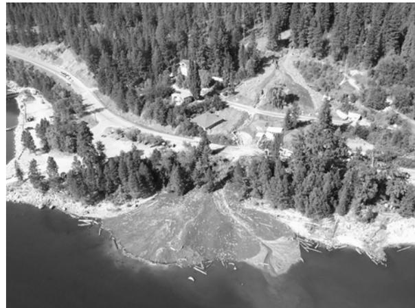
Figure 2. Kuskonook Creek fan following the debris flow of August 6, 2004.
