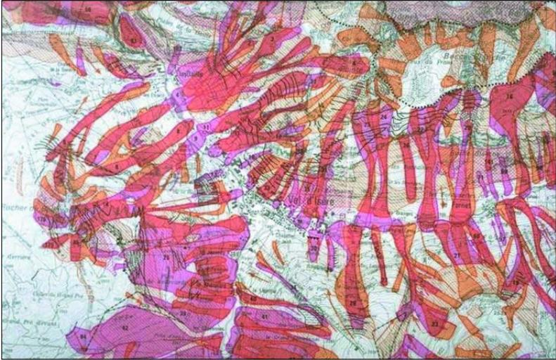
FIGURE 87 *Avalanche mapping for Val d'Isère, France (scale 1:25 000). Mapping in orange is from air photo interpretation. Mapping in magenta is based on field surveys, interviews with local witnesses including Forest Service rangers, and ski patrollers. Solid cross-hatching implies more certainty than areas delineated with broken cross-hatching. (After Borrel 1992)*
