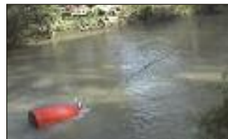
A sling pump operates on stream energy. Its propeller (impeller) is turned by water flow in the stream.
