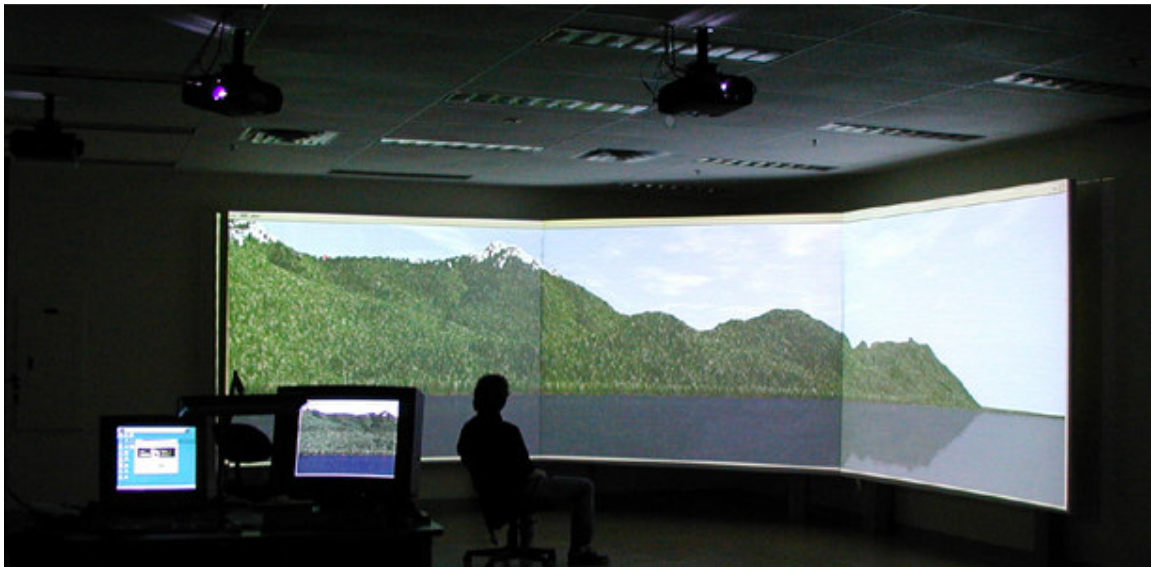
Figure 1: Landscape Immersion Laboratory LIL facility with a subject sitting in the target area (or “sweet spot”), reproducing a 120-degree angle of view with a panoramic image.
