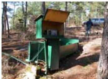
pumping samplers. Each sample was analyzed for total suspended sediment in a lab. Sediment and flow data and trapped coarse sediment were used to calculate total erosion for each storm. A siphoning recording rain gage was located at the sites for calculation of rainfall amounts and intensities.
