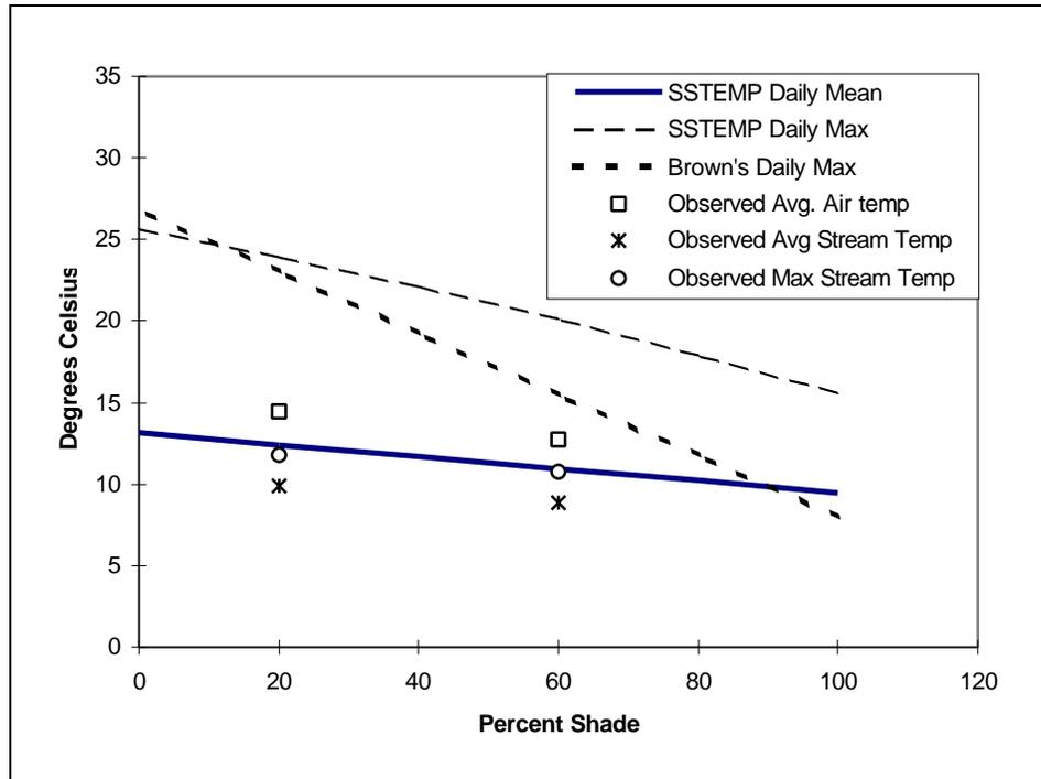
FIGURE 2. Observed stream temperatures at upstream (60 percent shade) and downstream edges (20 percent shade) of a clearcut compared with temperatures at bottom of clearcut predicted by two models. The points for comparison are the three daily maxima at 20 percent shade.
