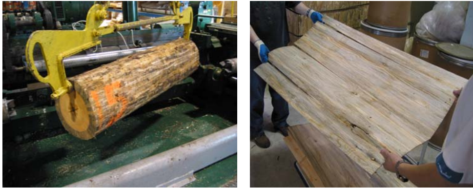
Figure 5. Pilot plant scale-up peeling test with a 1.2 m lathe
