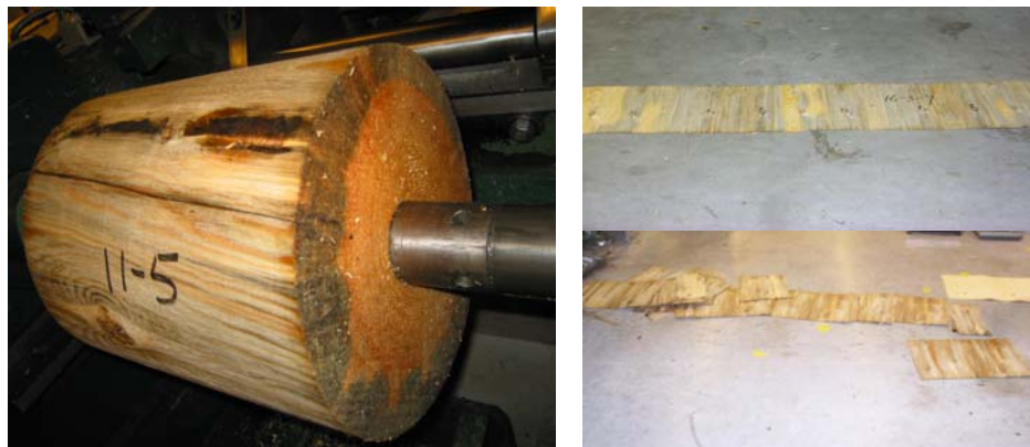
Figure 4. The 38-cm veneer mini-lathe (left) and veneer ribbon (right) peeled from beetle-killed logs
