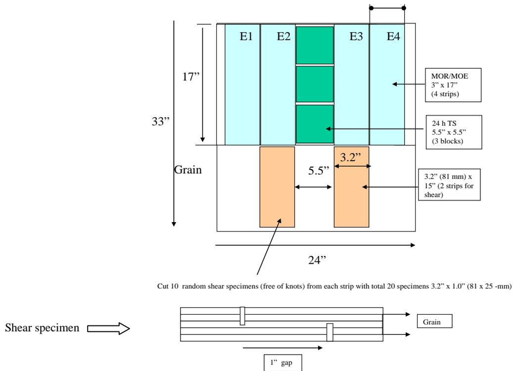
**Figure 3: The cutting diagram for 5-ply plywood**
