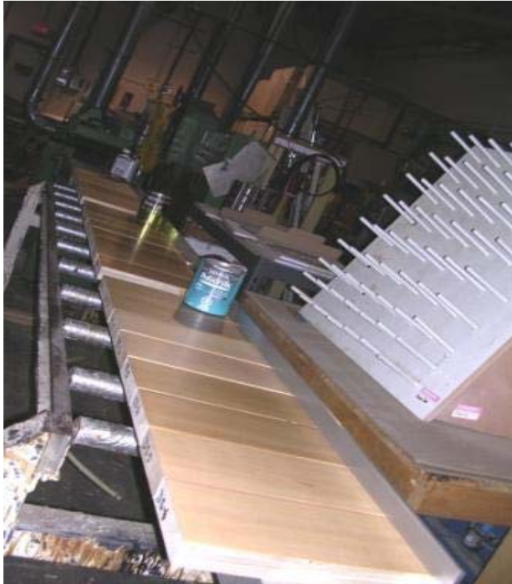
Figure 9 – Finish Acceptance Samples After One Coat
