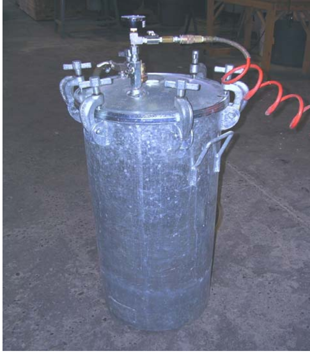
Figure 5 –Pressure Vessel Used in Vacuum-Pressure Testing
