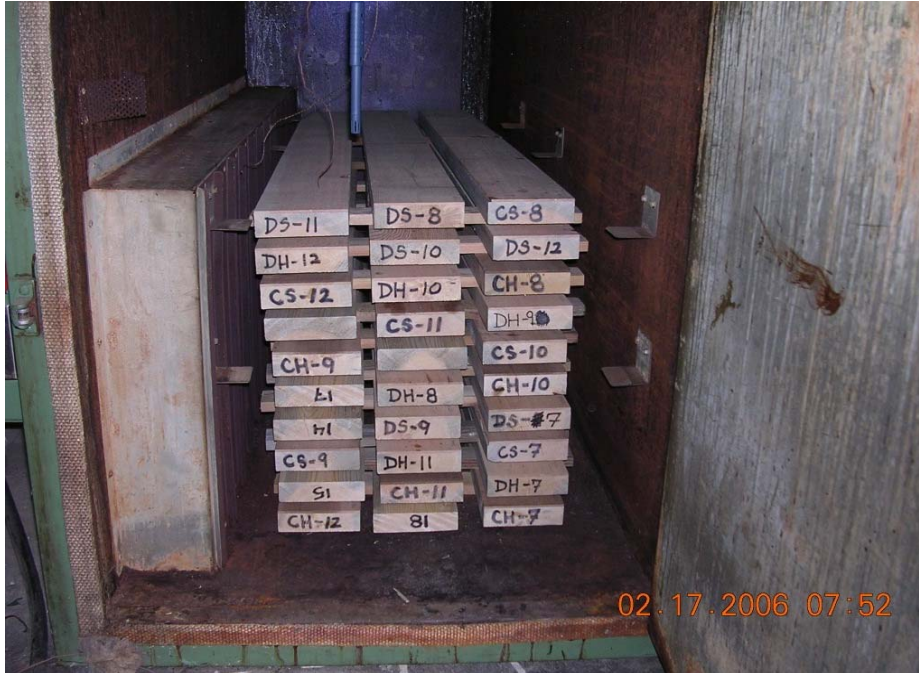
Figure 4 –Dimensional Stability Samples at Oven Conditions
