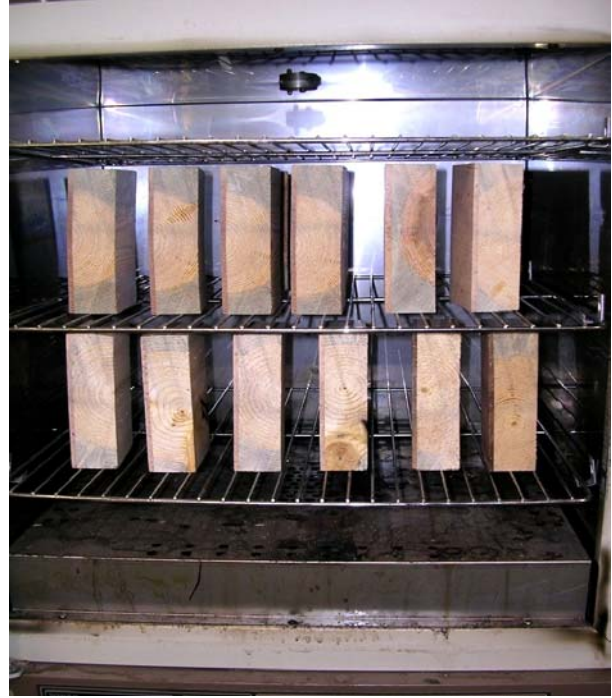
Figure 6 –Durability Samples in Drying Oven
