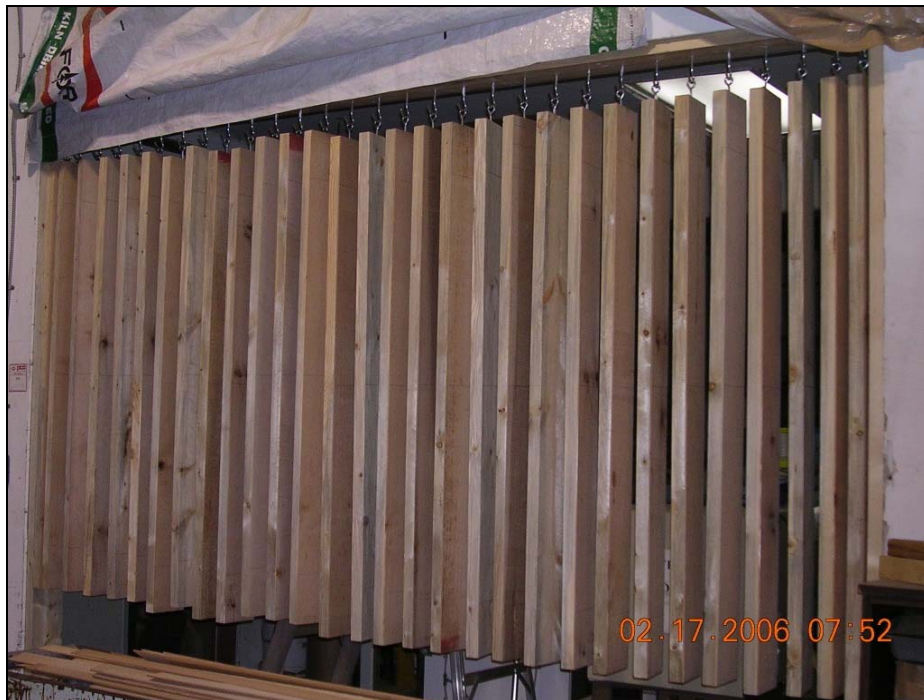
Figure 3- Dimensional Stability Samples Hung at Ambient Conditions
