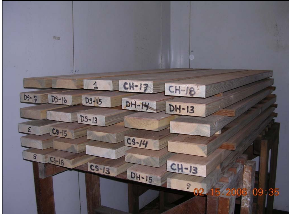
Figure 2 -Dimensional Stability Decking Samples At Forintek Humidity Chamber
