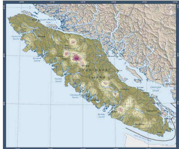
Figure 2. Density plot of 739 landslides on Vancouver Island between 2006 and 2007. Concentrations of landslides occurred in the Somerset range east of Cowichan Lake and west of the Alberni Inlet, and north of Gold River. These concentrations may now be analyzed against precipitation and wind data.
