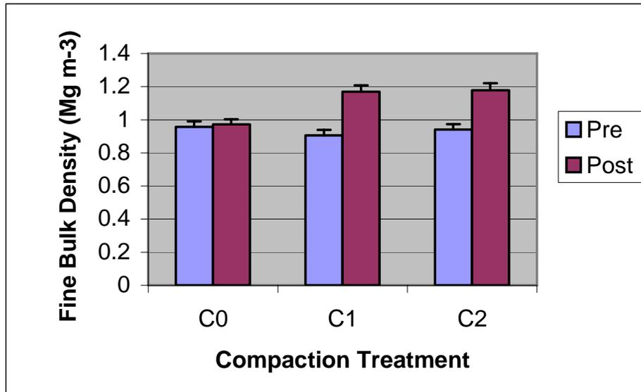
**Figure 22.** Mean pre- and post-treatment fine soil (<2mm) bulk density of the 0 – 20 cm soil layer for compaction treatments at the three Kamloops LTSP sites. Error bars are standard error of the mean.
