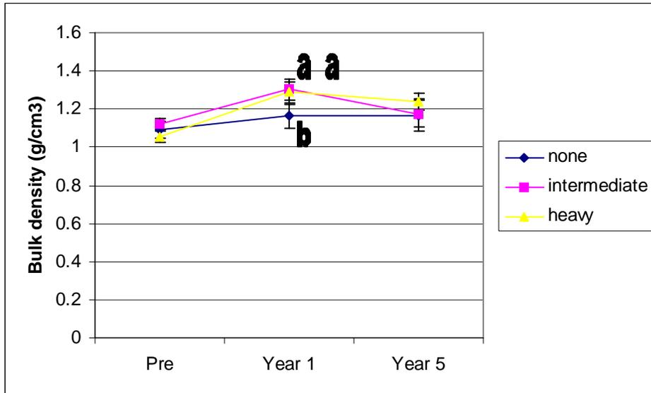
**Figure 2.** Lower (10-20 cm) mineral soil bulk density for the BWBS compaction treatments. Treatment means followed by the same letter do not differ significantly at  $p \leq 0.05$ .
