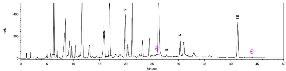
Fig. E-6. Ethyl acetate extract Soxhlet: 1- plicatic acid, 2- nezukone, 3-  $\gamma$  thujaplicin, 4-  $\beta$  thujaplicin, 5-  $\beta$  thujaplicinol, 6- thujic acid, 7- methyl thujate, IS- internal standard
