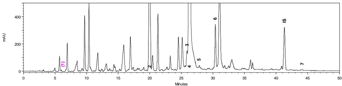
Fig. E-4. Dichloromethane extract: Soxhlet: 1- plicatic acid, 2- nezukone, 3-  $\gamma$  thujaplicin, 4-  $\beta$  thujaplicin, 5-  $\beta$  thujaplicinol, 6- thujic acid, 7- methyl thujate, IS- internal standard
