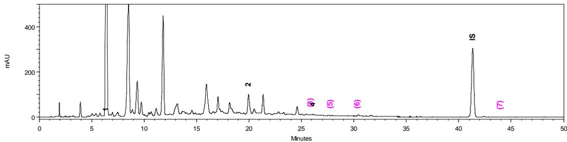
Fig. E-11. Water extract ultrasonic: 1- plicatic acid, 2- nezukone, 3-  $\gamma$  thujaplicin, 4-  $\beta$  thujaplicin, 5-  $\beta$  thujaplicinol, 6- thujic acid, 7- methyl thujate, IS- internal standard
