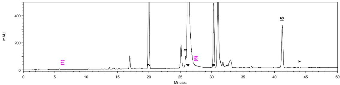
Fig. E-1. Hexane extract ultrasonic: 1- plicatic acid, 2- nezukone, 3-  $\gamma$  thujaplicin, 4-  $\beta$  thujaplicin, 5-  $\beta$  thujaplicinol, 6- thujic acid, 7- methyl thujate, IS- internal standard
