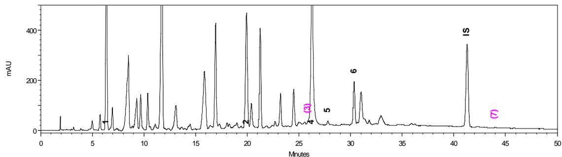
Fig. E-7. Ethanol extract ultrasonic: 1- plicatic acid, 2- nezukone, 3-  $\gamma$  thujaplicin, 4-  $\beta$  thujaplicin, 5-  $\beta$  thujaplicinol, 6- thujic acid, 7- methyl thujate, IS- internal standard
