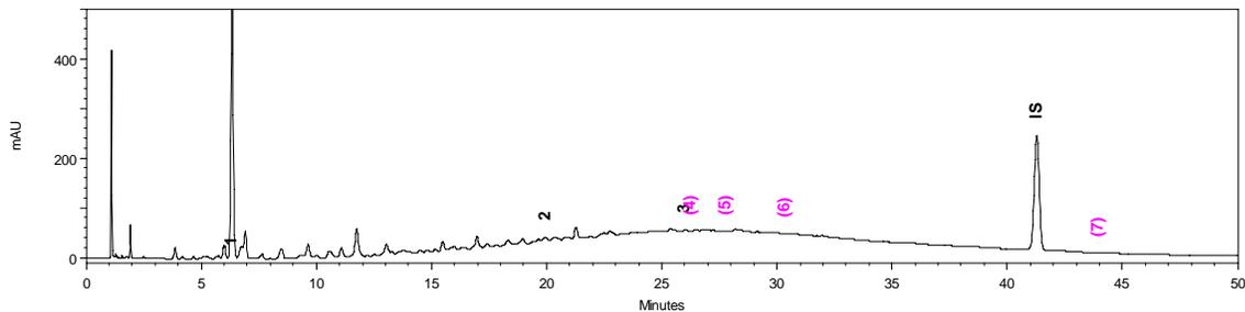
Fig. E-12. Water extract Soxhlet: 1- plicatic acid, 2- nezukone, 3-  $\gamma$  thujaplicin, 4-  $\beta$  thujaplicin, 5-  $\beta$  thujaplicinol, 6- thujic acid, 7- methyl thujate, IS- internal standard
