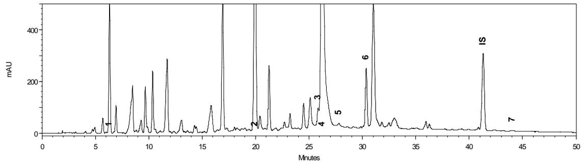
Fig.E-5. Ethyl acetate extract ultrasonic: 1- plicatic acid, 2- nezukone, 3-  $\gamma$  thujaplicin, 4-  $\beta$  thujaplicin, 5-  $\beta$  thujaplicinol, 6- thujic acid, 7- methyl thujate, IS- internal standard
