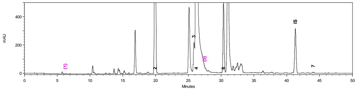
Fig. E-2. Hexane extract Soxhlet: 1- plicatic acid, 2- nezukone, 3-  $\gamma$  thujaplicin, 4-  $\beta$  thujaplicin, 5-  $\beta$  thujaplicinol, 6- thujic acid, 7- methyl thujate, IS- internal standard
