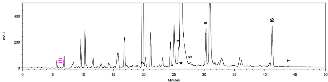
Fig. E-3. Dichloromethane extract ultrasonic: 1- plicatic acid, 2- nezukone, 3-  $\gamma$  thujaplicin, 4-  $\beta$  thujaplicin, 5-  $\beta$  thujaplicinol, 6- thujic acid, 7- methyl thujate, IS- internal standard
