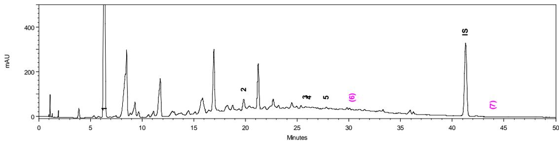
Fig. E-10. Methanol extract Soxhlet: 1- plicatic acid, 2- nezukone, 3-  $\gamma$  thujaplicin, 4-  $\beta$  thujaplicin, 5-  $\beta$  thujaplicinol, 6- thujic acid, 7- methyl thujate, IS- internal standard
