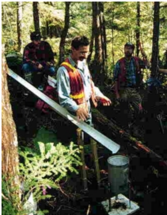
FIGURE 2. Troughing for monitoring throughfall and canopy drip.
