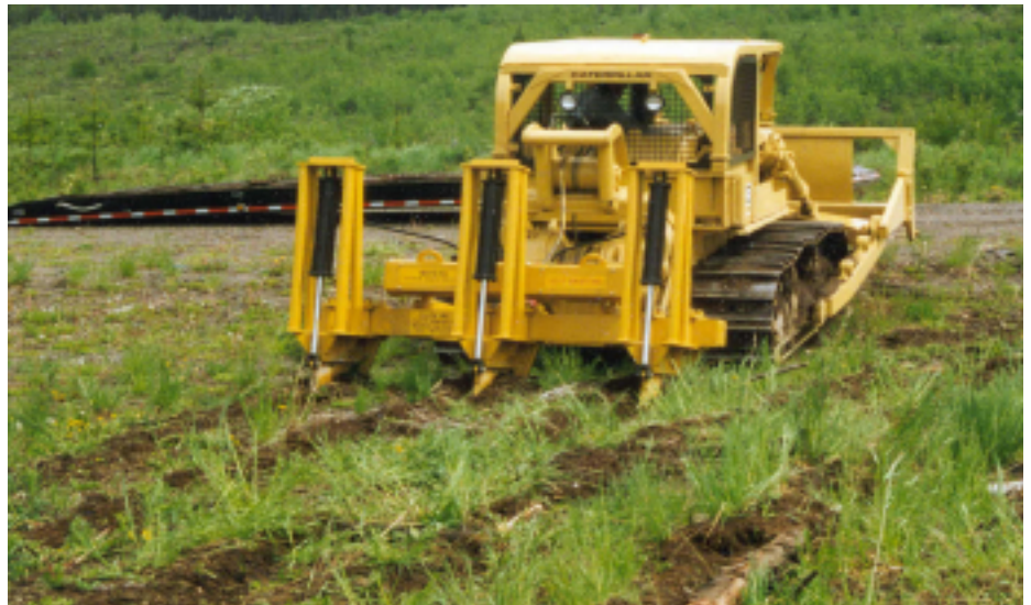
Figure 1. The winged subsoiler in action.
