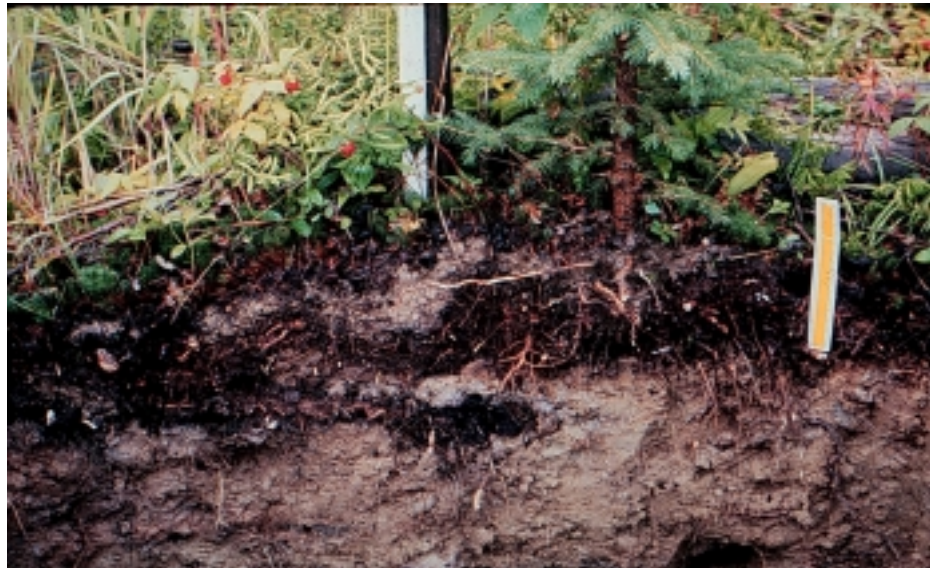
Figure 1. Cross-section of mound showing buried organic layer and mineral cap
