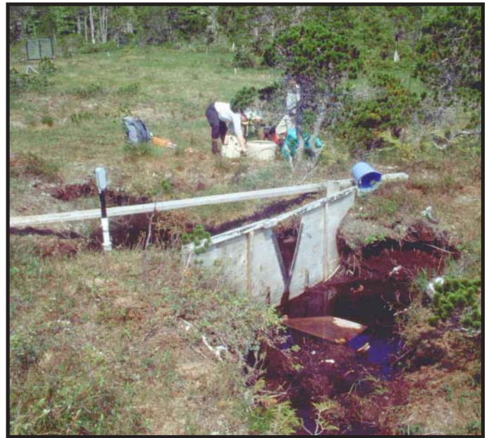
Figure 3. Bog stream weir. 60° v-notch weir measures discharge on bog stream. Note stage recorder to left behind the weir.
