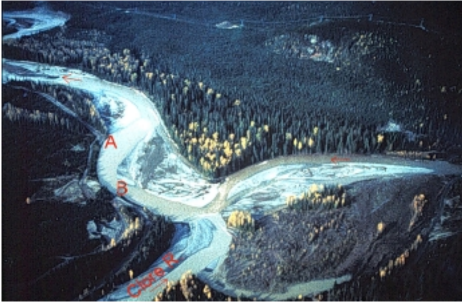
Figure 2. Clore River confluence. During the 1978 flood, 300 metres of the Copper River Road were eroded (between point A and B).
