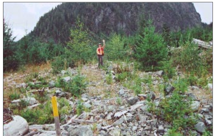
Figure 7. Plot N80 showed low stocking levels of Douglas-fir, but trees that had become established were growing well. A high content of coarse fragments in the road substrate, combined with poor decompaction, likely contributed to poor survival on this site.
