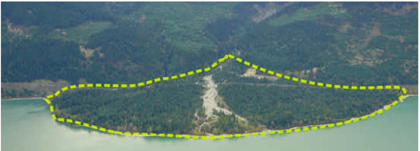
Figure 4. An alluvial fan, with the boundaries of the fan outlined in yellow.
