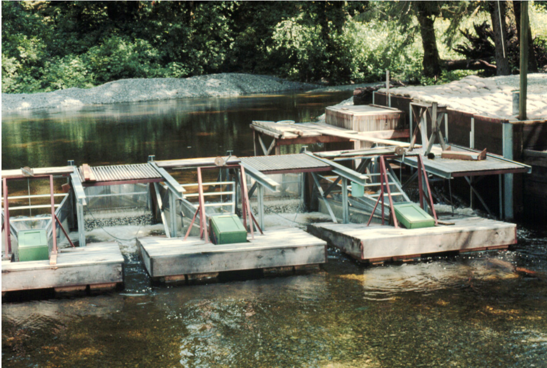
Carnation Creek fish fence (looking upstream). The fence is configured with fan traps and trap boxes (green) for collecting seaward migrating juveniles in spring (early February to mid-June).
