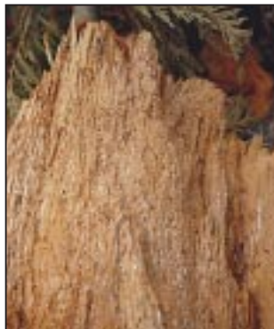
White rot – This pitted type of decay is common to many white rots.
