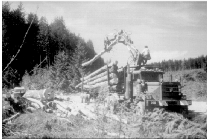
Figure 110 The self-loading log truck can operate anywhere the truck can drive. Self-loaders can pick up scattered loads without the expense of moving a loader.
