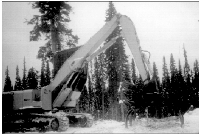
Figure 107 A hydraulic loader equipped with a shortwood log grapple. This grapple does not require a “heel” because the logs are short and easy to balance.
