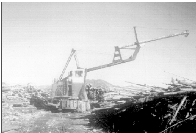
Figure 109 A rubber-mounted line loader. This type of carrier provides more mobility than tracked designs.
