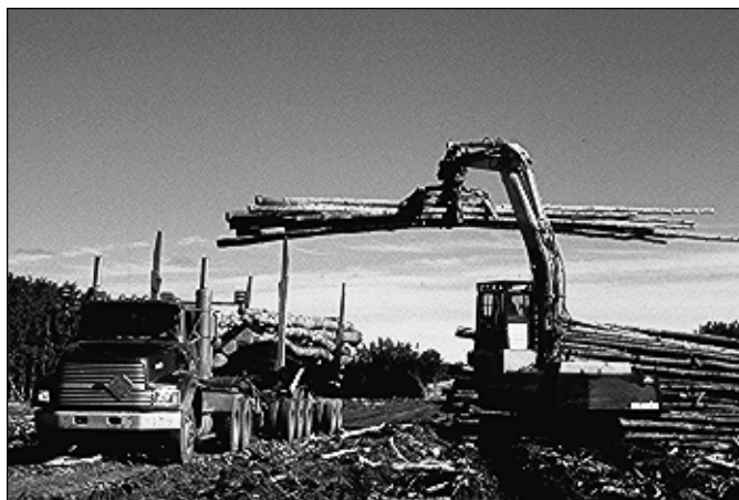
Figure 108 A hydraulic “butt ‘n top” loader in a roadside operation. The butt ‘n top can load trucks from the side, and turn the logs end-for-end as required.
