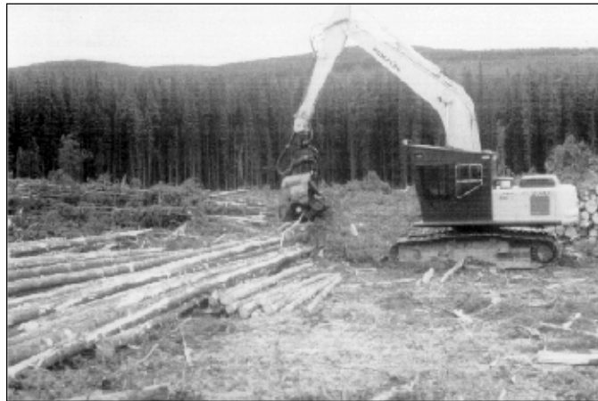
Figure 97 A dangle-head processor working at roadside in a typical, small-diameter stand appropriate for this type of equipment.
