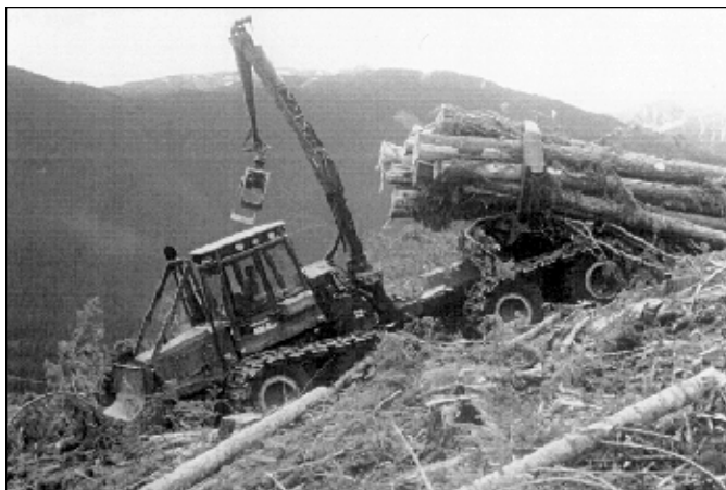
Figure 3 Clambunk skidders may be able to work on the steeper slopes of the new operating area.
