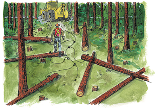
Poorly set turns will hang up on leave trees.
