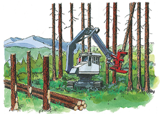
When using feller bunchers, stubs can safely be left for wildlife habitat.
