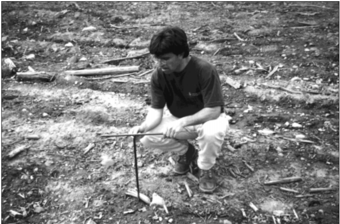
FIGURE 10 Evaluating tillage depth (Morice Forest District, Telkwa River Forestry Road, km 15). The indicated depth of loosened soil is approximately 40 cm (total length of probe is 1 m), indicating effective tillage with a winged subsoiler.
