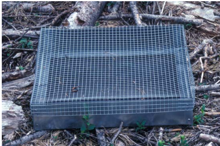
FIGURE 2 50 \times 50 cm metal seedfall trap.
