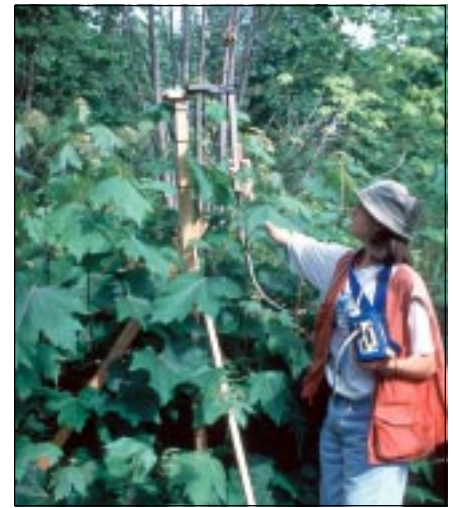
figure 2 Plant canopy analyzer (LAI-2000) used to record light measurements next to a quantum sensor.
