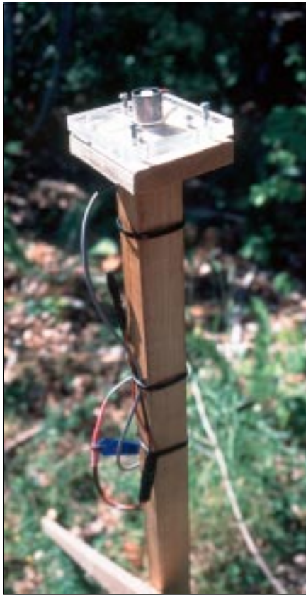
figure 3 Quantum sensor positioned on top of a two metre wooden stake.
