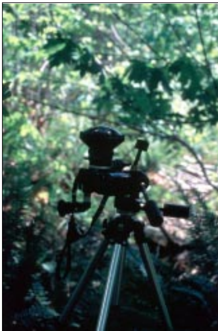
figure 4 Camera set-up for hemispherical (fish-eye) photography.
