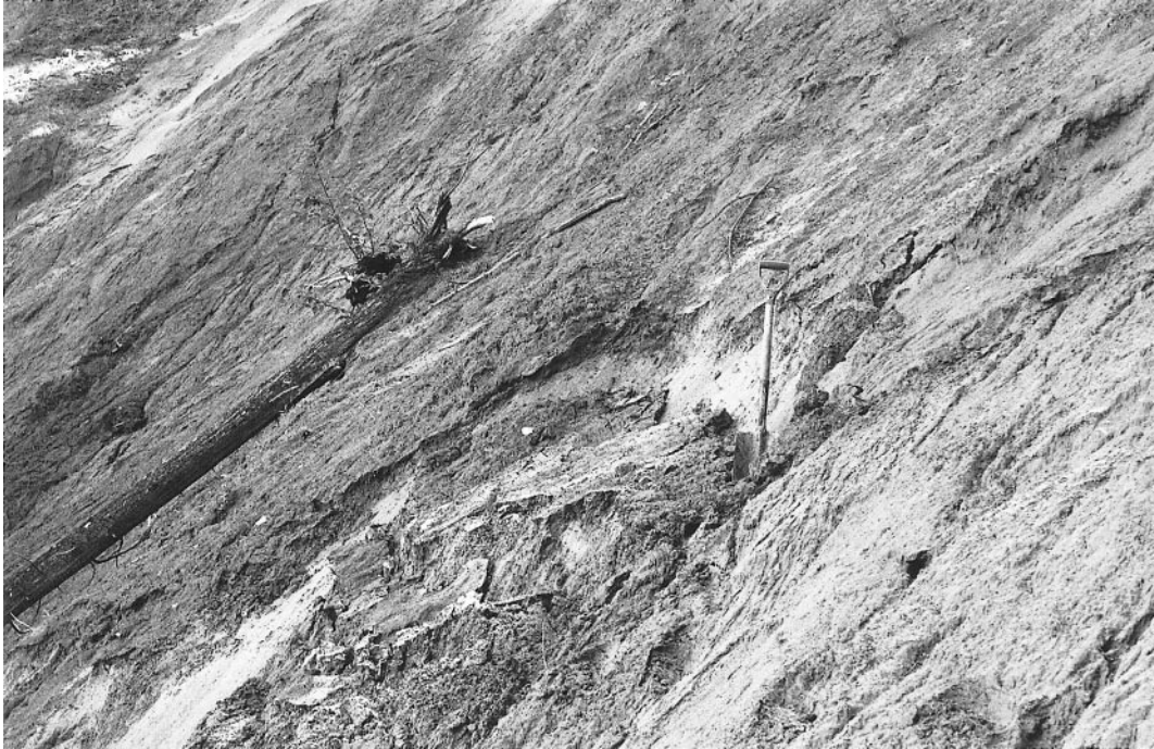
Fig. 5. Slide 66044:01 (see Fig. 2 for location). Approximate depth of rupture surface for slide shown in Fig. 4. One metre long shovel for scale.
