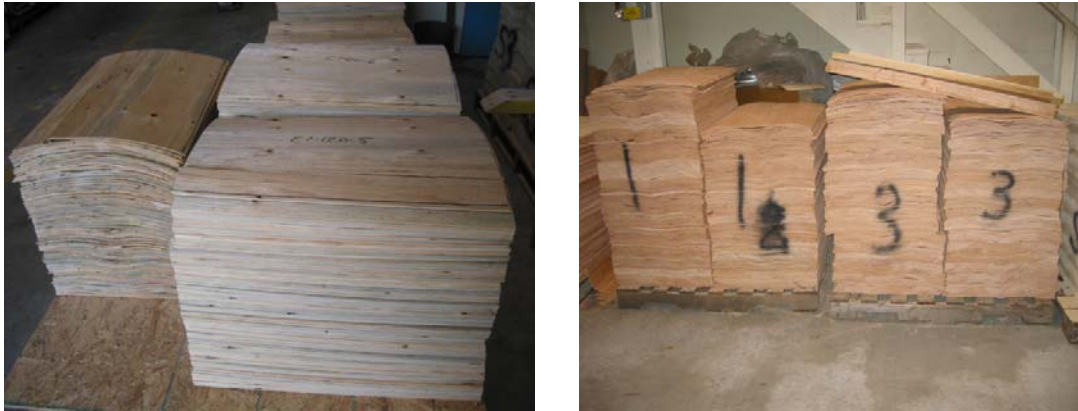
Figure 2: Preparation of the MPB and Douglas-fir veneer for plywood manufacturing
