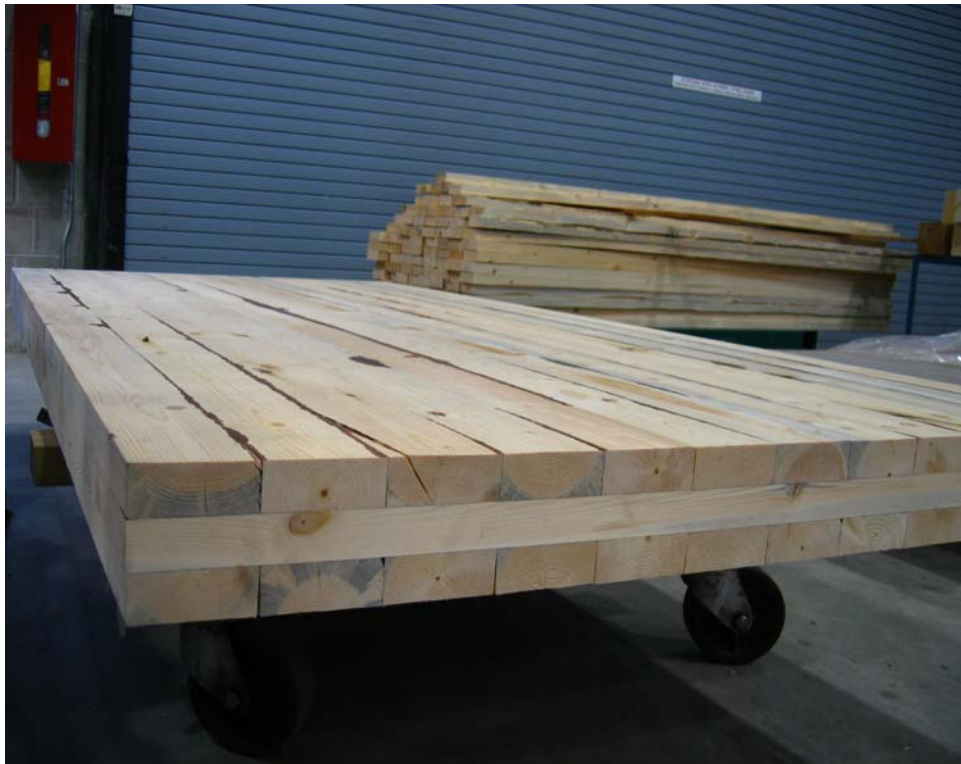
Figure 21. 3-layer glued cross laminated MPB wood plate.
