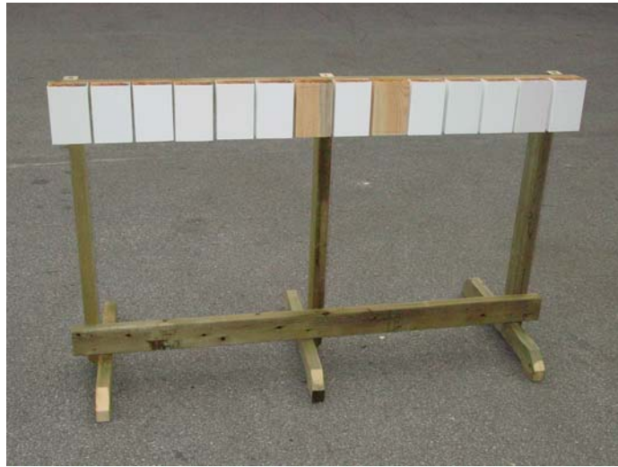
Figure 2. One of four test fences used to expose painted blue-stained samples to the weather
