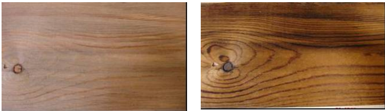
Figure 12 Sample 16-2, 2 hours' treatment, blue and brown-stain were masked
