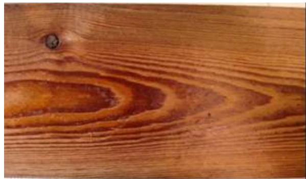
Figure 15 Sample 3-2, 2 hours' treatment, oil residue on the surface of the treated board
