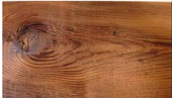
Figure 14 Sample 10-2, 2 hours' treatment, tight knots survived during the treatment
