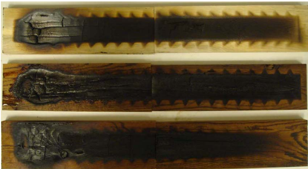
Figure 25 Flame spread pattern on untreated pine, oil thermally-treated pine and double-treated pine with oil-thermal treatment and fire retardant treatment (three treatments from the top to the bottom) during the two-foot tunnel test
