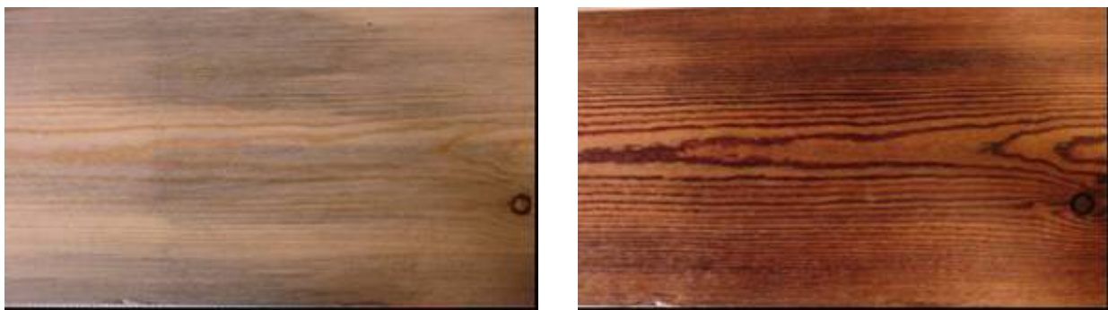
Figure 11 Sample 8-2, 2 hours' treatment, blue-stain was masked
