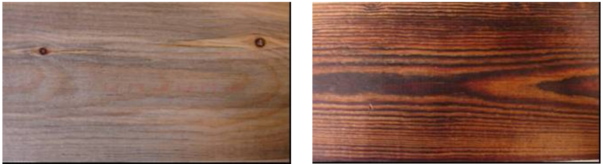
Figure 17 Sample 18-2, 2 hours' treatment, very high oil absorption
