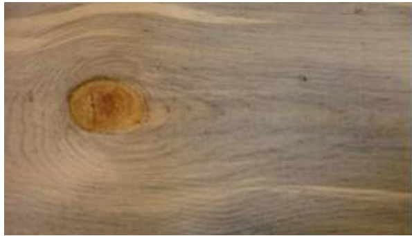
Figure 14 Sample 10-2, 2 hours' treatment, tight knots survived during the treatment
