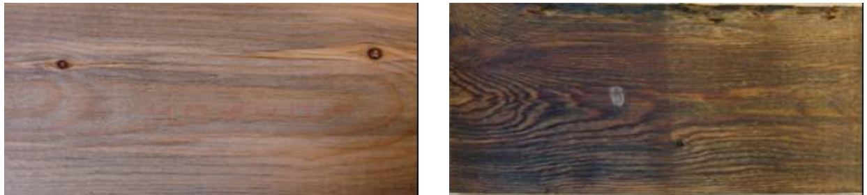
Figure 18 Sample 18-1, 1 hour's treatment, very high oil absorption
