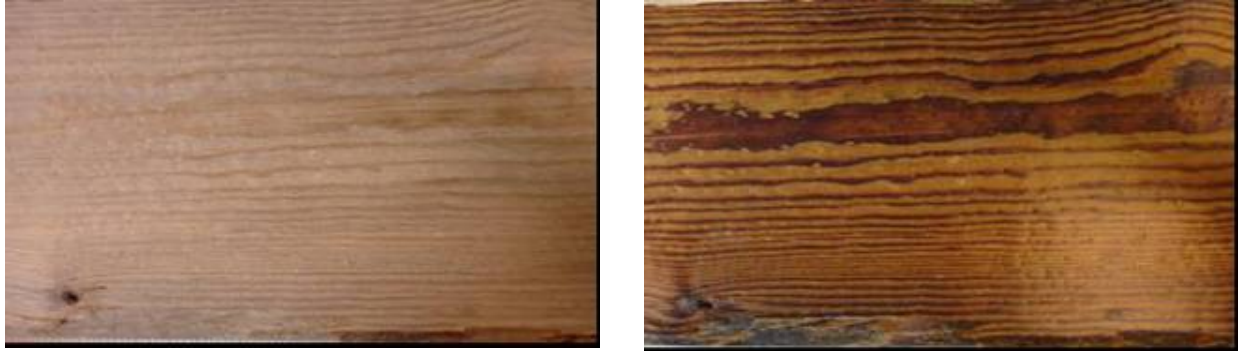
Figure 16 Sample 17-2, 2 hours' treatment, high oil absorption
