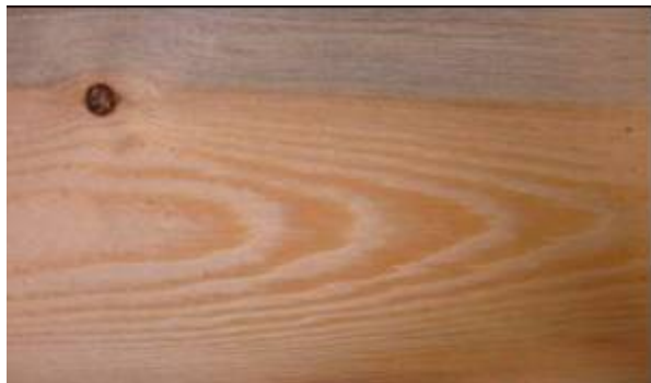
Figure 15 Sample 3-2, 2 hours' treatment, oil residue on the surface of the treated board
