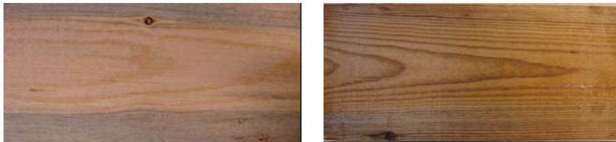
Figure 19 Sample 9-1, 1 hours' treatment, blue-stain was still visible
