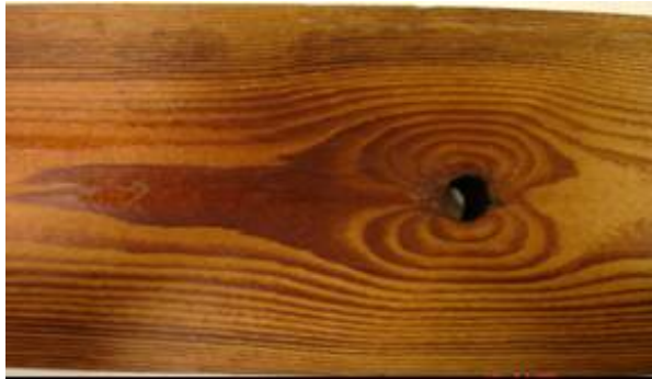
Figure 13 Loose knots were missing after 2 hours' oil-thermal treatment
