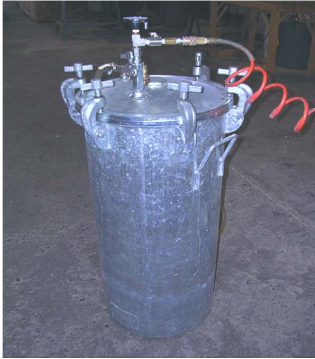
Figure 5 –Pressure Vessel Used in Vacuum-Pressure Testing
