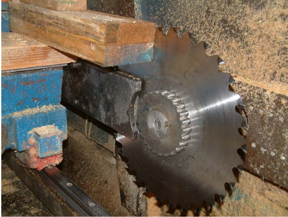
Photo 3.1 Details of guided saw and height of cant with respect to the saw
