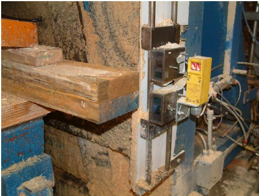
Photo 3.2 Laser probes used to measure surface deviation on cut board
