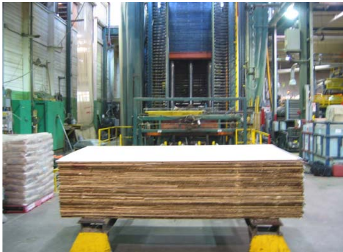
Figure 8: Forty 5-ply Douglas-fir plywood panels unloaded from the press
