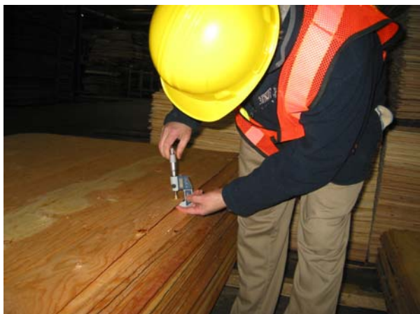
Figure 10: Measurement of Douglas-fir dry veneer thickness
