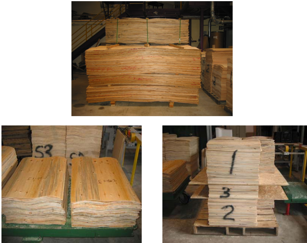
Figure 1: Preparation of sample veneer sheets for plywood/LVL manufacturing
