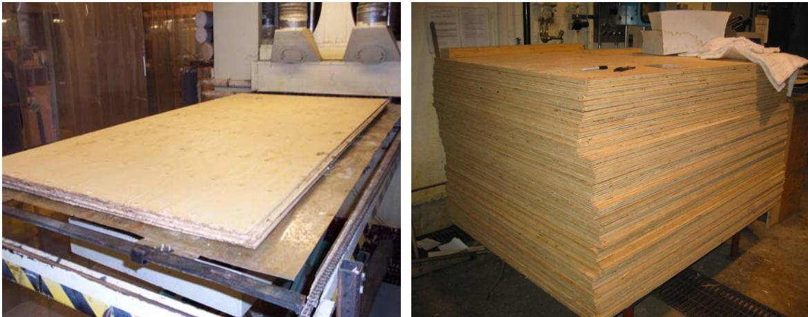
Figure 5: Full-size plywood/LVL manufacturing on ARC's 4'x 8' press
