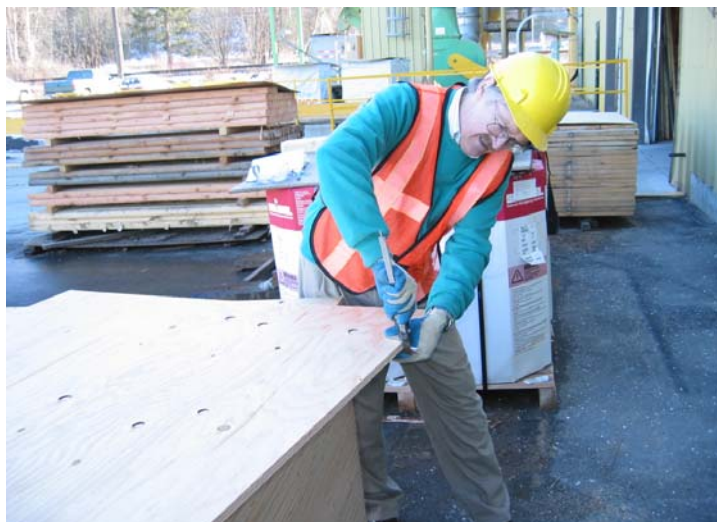
Figure 9: Measurement of 5-ply Douglas-fir plywood thickness
