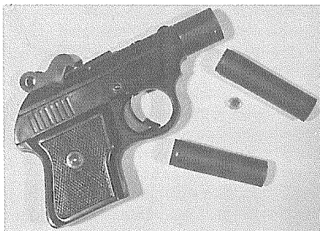
Fig. 8 Orchard and vineyard pistol with blank cap and shells
