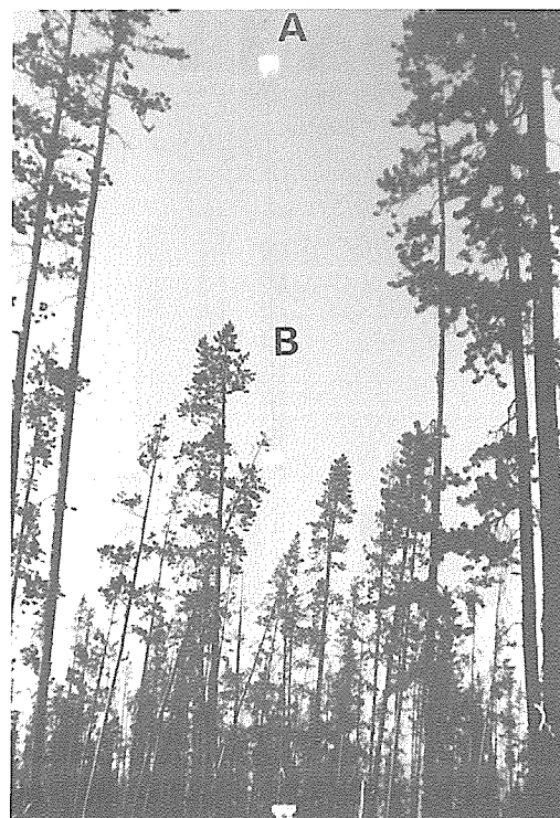
Figure 3--Omnidirectional passive barrier traps used to catch flying beetles: (A) horizontal support line with pulley for attachment of vertical line; (B) vertical line used to raise and lower traps, with three traps attached.
