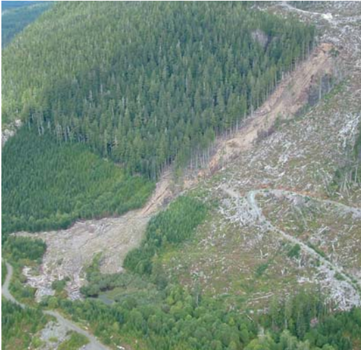
Figure 2. A landslide related to logging and road drainage in a recent block. The post-Code rate of landslides appears to have been reduced (from pre-Code) by increased buffers around streams, escarpments and gullies, better road construction and increased reliance on geoscientists and engineers. Photo added by R. Guthrie.
