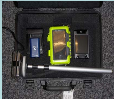
Figure 2. The basic equipment for a range inspection includes a PDA, a GPS, a telescopic pole, protective cases and an extended battery.
