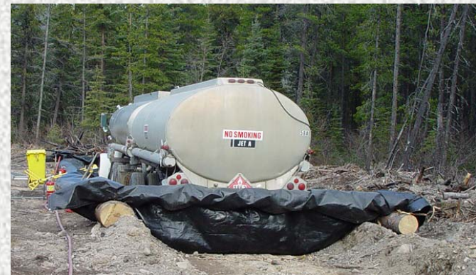
Heavy duty tarp berm
