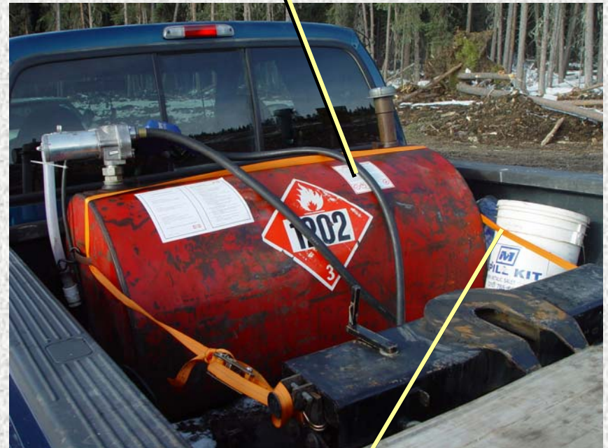
Unacceptable securing method
