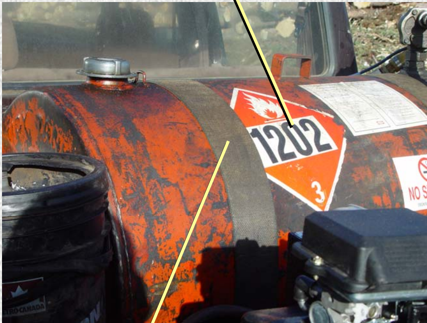
Well secured non-spec tank
